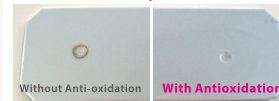
Without Anti-oxidation With Antioxidation The process for removing burn marks on the welded side can be eliminated.
